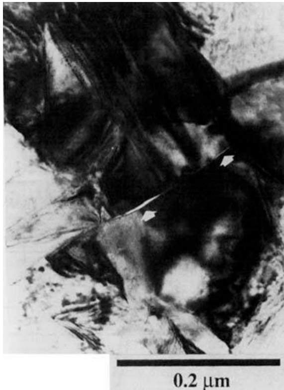
Fig. 7.35 TEM micrograph of 3Y-TZP after fatigue shows a lenticular microcrack along the grain boundary (as indicated by arrows ) [19]. With kind permission of John Wiley and Sons
