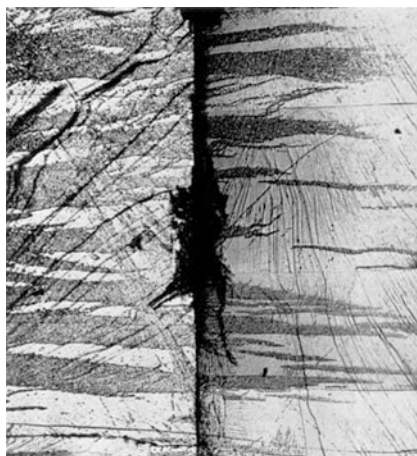
Fig. 2.37 a Etched grains of polycrystalline MgO deformed at room temperature, X95; b deformed at 1240 °C, X95; c deformed at 1240 °C, X190 [23]. With kind permission of Elsevier
