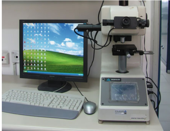
Fig. 1.55 Buehler made a combined hardness tester for Vickers, Knoop and Rockwell. Model #1600-6400. Load range 1–2000 g
