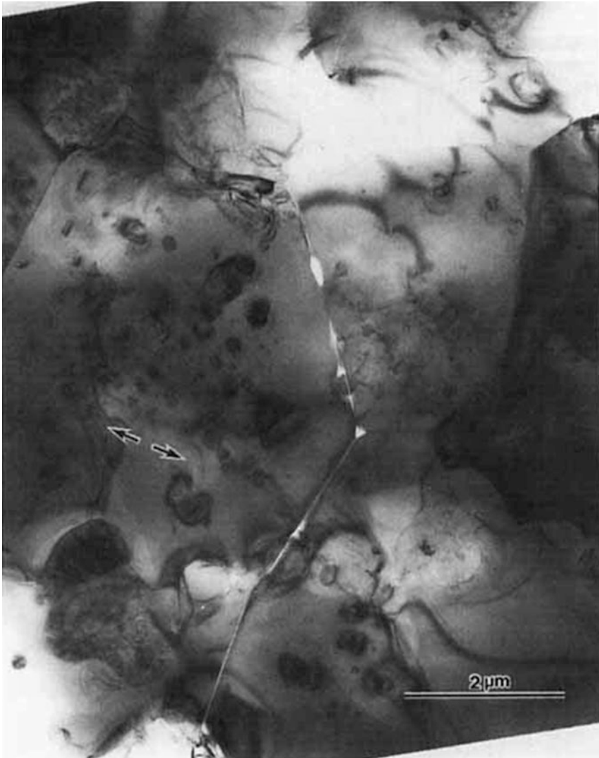
Fig. 9.35 Transmission electron micrograph of a trace of intergranular crack propagation. The sample was tested at 1200 °C and 100 MPa in tension. Note the transgranular-fractured nanoparticle. The stress direction is indicated by an arrow [23]. With kind permission of John Wiley and Sons
