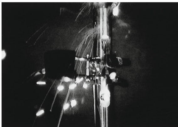
Fig. 3.17 Photo showing the moment of fracturing a BAA 11 specimen tested at room temperature in air [32]. With kind permission from Springer Science+Business Media B.V.
